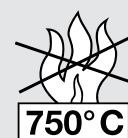
Burning behaviour: Glow wire test according to IEC 60 695-2-1: 750 °C, flame-retardant, self-extinguishing
