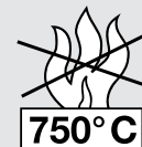
Burning behaviour: Glow wire test according to IEC 60 695-2-1: 750 °C, flame-retardant,
